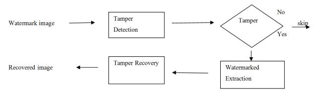
Block Diagram1: Tamper Detection
